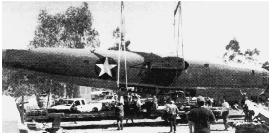
The Liberator's 66.4-foot-long fuselage being lowered onto flatbed trailer for the trip to Utah.
